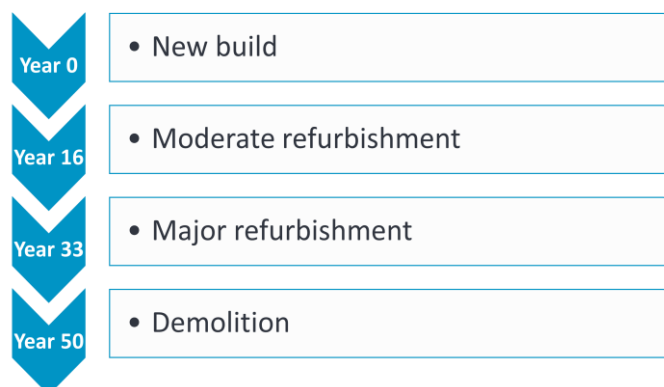
Figure 10 Building-refurbishment-demolition cycle of health infrastructure
